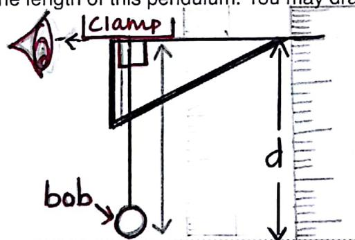
Fix the set square exactly where the string begins. Place a ruler at the other end of the set square as shown. View from the left of the set-up and mark off the measure [1]
