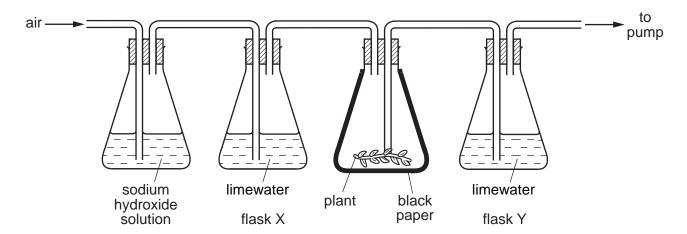
Sodium hydroxide removes carbon dioxide from the air. Limewater goes cloudy if carbon dioxide is bubbled through it.
