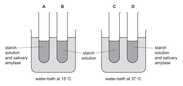
11 An experiment was carried out using the apparatus shown.
