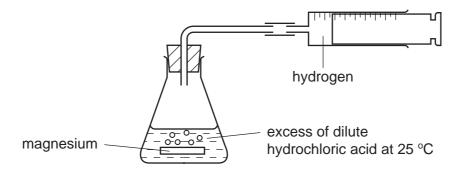
Increasing the concentration of the acid and increasing the temperature both affect the speed of reaction.
