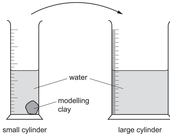
The reading on the small measuring cylinder goes down by  $20 \text{ cm}^3$ .
