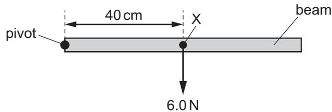
The beam weighs 6.0 N and its weight acts at a point X 40 cm from the pivot.
