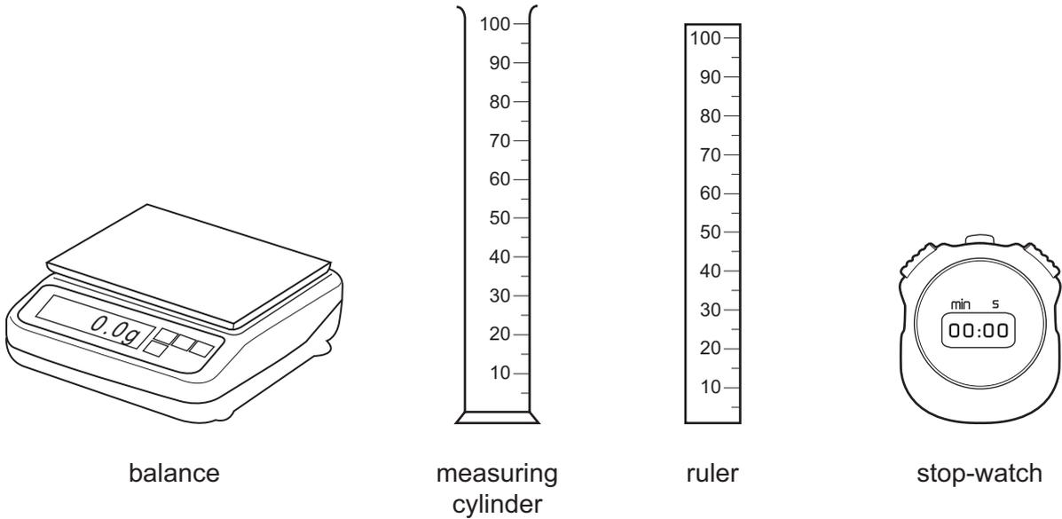
Which pieces of apparatus are used to find the density of a liquid?
