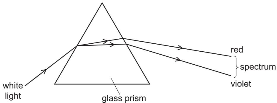
The spectrum can be seen emerging from the prism.
