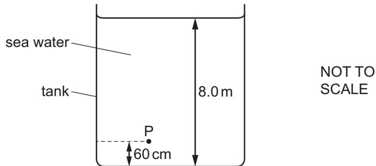
The density of the sea water is  $1020 \text{ kg/m}^3$ .
