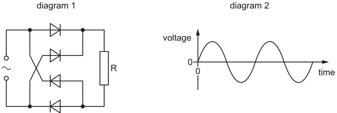
Which graph correctly shows the voltage–time curve across resistor R?
