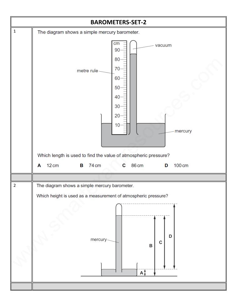
The diagram shows a simple mercury barometer, used to measure atmospheric pressure.
