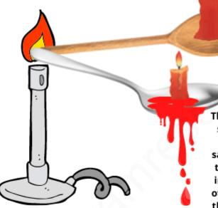
The candle in the metal spoon keeps burning normally but at the same time, wax is seen to melt and drip. This indicates that the end of the spoon that holds the candle has become hot due to conduction and that metal is a good conductor
