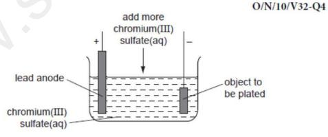
This is because the electrolyte is getting used up. The ions lost at the cathode are not being replaced by the anode.
