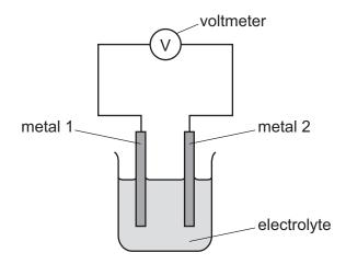
The simple cell was used with different metals as electrodes. The voltages were recorded in the table.
