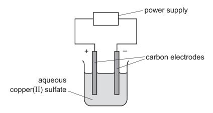
Oxygen gas forms at the positive electrode (anode).
