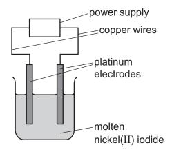
During electrolysis, charge is transferred through the copper wires and through the molten nickel(II) iodide.
