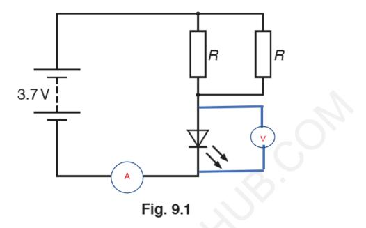
The normal operating voltage of the LED is 2.1 V and the normal current is 0.19A.
