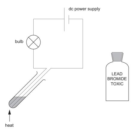
The lead bromide was heated until molten. A brown gas was given off.
