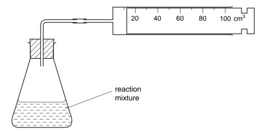
The volume of hydrogen collected at one minute intervals was measured. Use the diagrams to record the volumes in the table.
