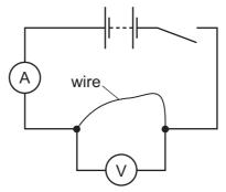
When the switch is closed, the ammeter reads 2A and the voltmeter reads 10V.
