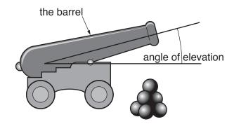
The range depends on the angle of elevation.
