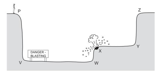
After the explosion, she hears two bangs. One bang is heard a fraction of a second after the other. The second bang is an echo.
