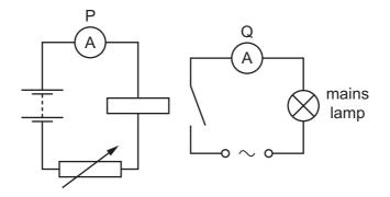
The variable resistor is used to vary the current in the relay coil. The mains lamp switches on when there is a large enough current in the relay coil.
