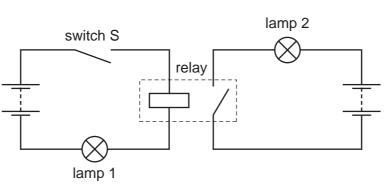
When switch S is closed, the relay operates. What is the state of the lamps?
