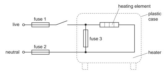
Which of the fuses are correctly placed?
