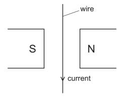
The magnet and current cause a force to act on the wire.
