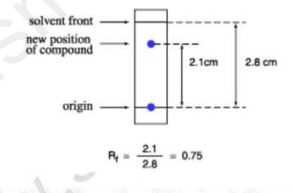
The R<sub>f</sub> value of a sample = <u>distance travelled by sample</u> distance travelled by solvent front
