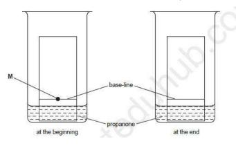
The reason is that if the solvent is above the base line, the dyes would get washed off in the solvent( or in other words, they would dissolve in the solvent)
