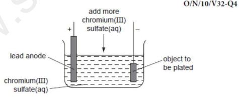
This is because the electrolyte is getting used up. The ions lost at the cathode are not being replaced by the anode.
