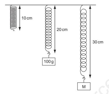
The extension of the spring is directly proportional to the mass hung on it.
