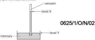
If atmospheric pressure increases, what happens to level X and to level Y?
