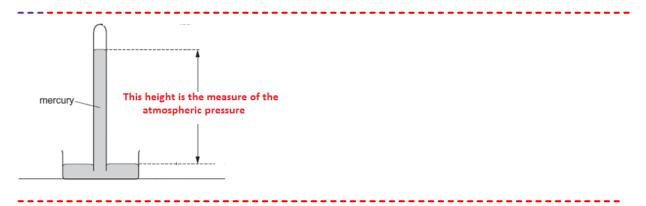
When the atmospheric pressure rises then the level of mercury at L rises and
