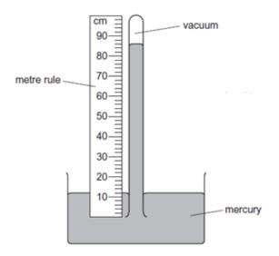
• It consists of an inverted glass tube containing mercury with its lower end under the surface of mercury in a container open to the atmosphere.
