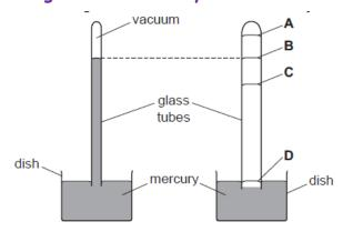
Imagine two mercury barometers standing side by side, then it does not matter what the diameter of the capillary tubes of the two barometers is, the mercury will stand at the same height as the height is the measure of the atmospheric pressure.
