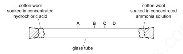
After ten minutes a white solid forms in the tube where the gases meet.
