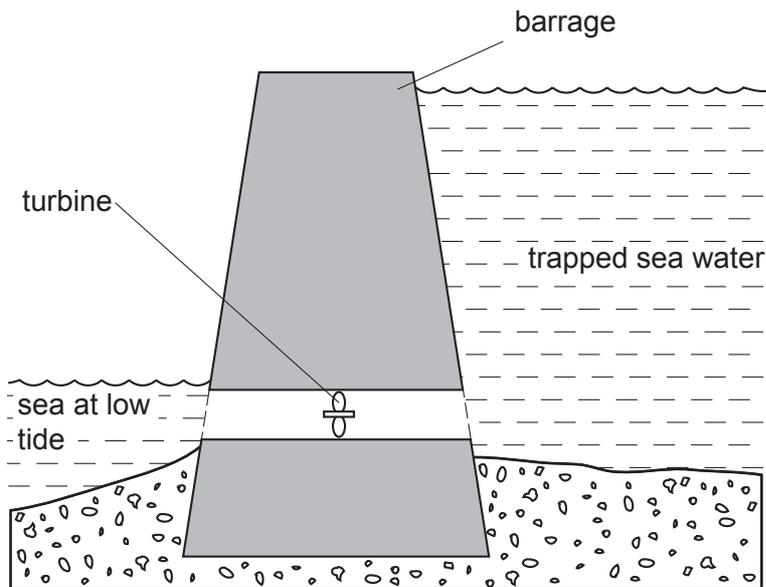
At low tide the water is allowed to flow back into the sea through a turbine.
