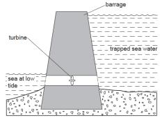
In a tidal power station, the potential energy is being converted to electrical energy
