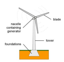
Wind turbines have huge blades mounted on a tall tower. The blades are connected to a nacelleor housing that contains gears linked to a generator. As the wind blows, it transfers some of its kinetic energy to the blades, which turn and drive the generator. A cable between the generator and the shore delivers the electricity to local users or via a network of cables to distant users. Several wind turbines may be grouped together in windy locations to form wind farms.
