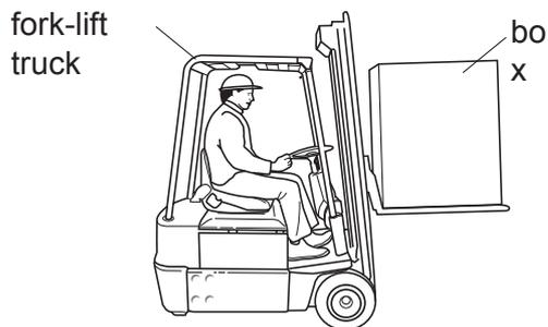
The force exerted by the fork-lift truck on the box is 3500 N upwards.
