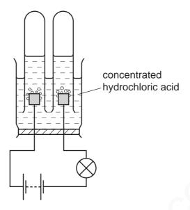
Bubbles were observed at both electrodes.
