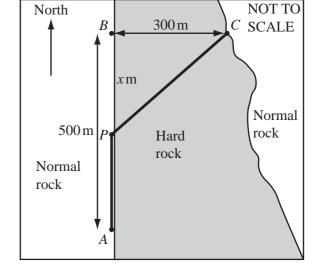
Through normal rock, from *A* to *P*, the drill moves forward at 2 metres per hour. Through the hard rock, from *P* to *C*, the drill moves forward at 1 metre per hour.
