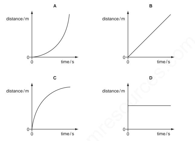
The graph shows the motion of a train during part of a journey. At which labelled point on the graph could the train be waiting at a station?
